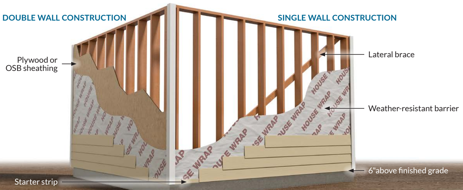
Double and Single Wall Construction
