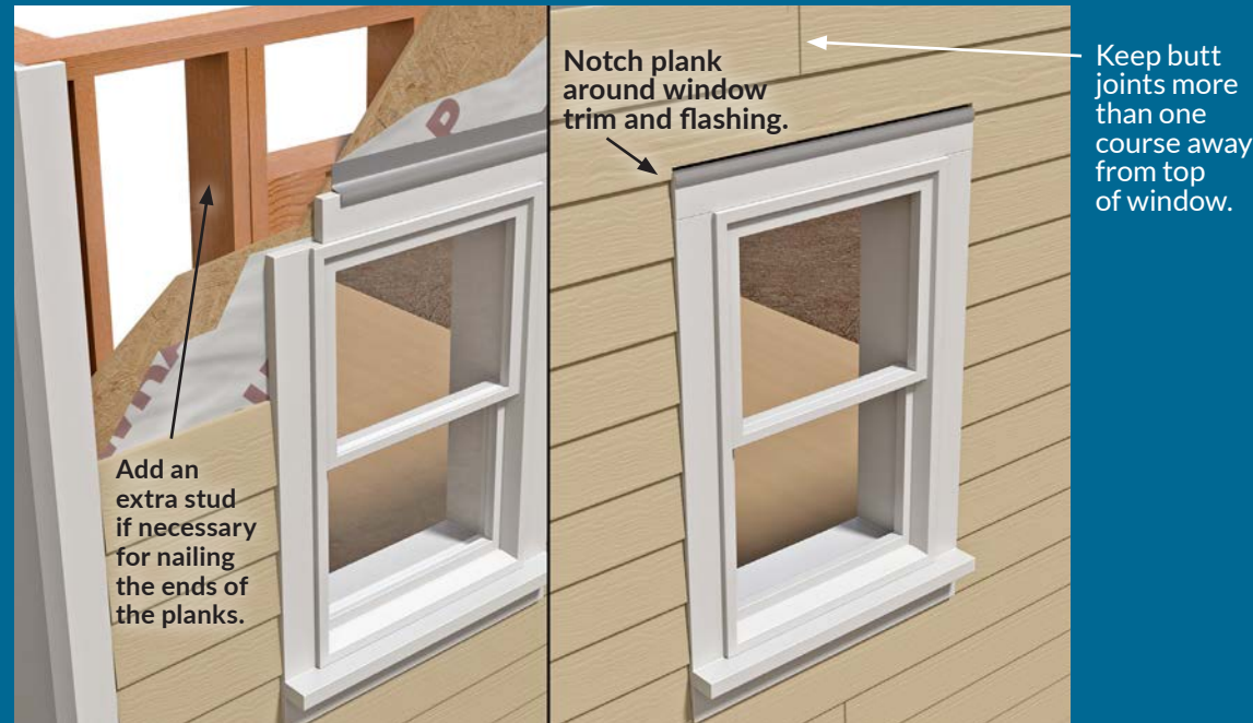
Planking around windows
